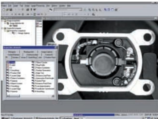
Example: completeness checking in the assembly of a motor; selecting the elements to check when creating a new project
