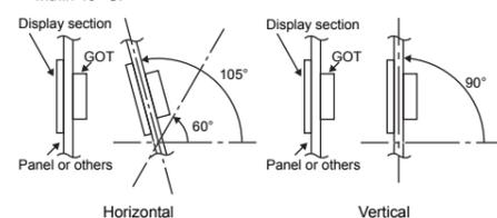
According to the dimensions in the following table, leave clearances between the GOT and the other devices. The values enclosed in square brackets apply to the case where no other equipment generating radiated noise (such as a contactor) or heat is installed near the GOT. However, keep the ambient temperature of the GOT to 55 °C or lower.
